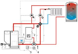
Hydraulic diagram with the reserve boiler and the 4-way valve in close circuit 1 – regulator, 2 – reserve boiler, 3 – U3 module, 2 pcs., 4 – switching valve servo (with limit switches) - to ensure free gravitational flow of water in the boiler circuit, active cross-section of switching valve (4) has to be larger than or equal to cross-section of boiler circuit pipes. Use pipes of large cross section for gravitational boiler circuit.
