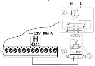
Connection of an external alarm annunciator 1 - regulator - module A, 2 - external alarm annunciator, 3 - relay RM 84-2012-35-1012 RELPOL and base GZT80 RELPOL.
