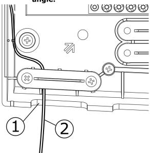
The output of the capillary: 1 - Cable opening 2 - The STB capillary cable, which was being correctly taken out from the clamp box.
