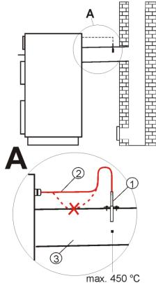
Connecting emission sensor: 1 – exhaust temp. sensor type CT2S, 2 – sensor lead, 3 – flue.
