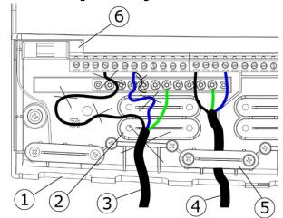
1 – cable outlets, 2 – holdfasts placing (should be broken out for the casing), 3 – improper cable connection (it is not allowed to coil excess of the cable inside the device and to leave cables with stripped insulation), 4 – proper cable connection, 5 – holdfast of the cable, 6 – connector.
