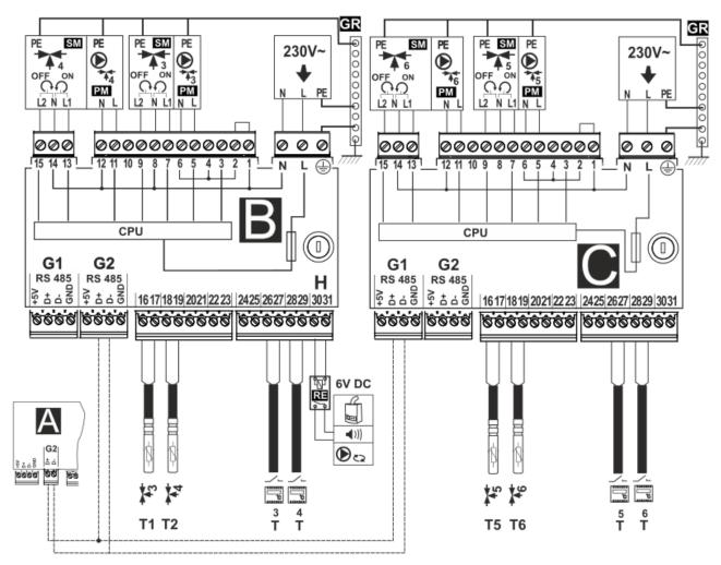
**Electric scheme – additional modules TIS TRONIC 61B and TIS TRONIC 61C**: **T1, T2** – mixer 3,4 temp. sensor type CT4, **T5, T6** – mixer 5,6 temp. sensor type CT4, **T** – room thermostat (ON-NC).
