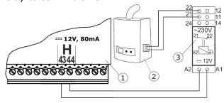
Model diagram of layout for connecting a reserve boiler to the regulator, where: 1- regulator, 2 - reserve boiler (gas- or oil-fired), 3 - module U3, consisting of relay RM 84-2012-35-1012 and base GZT80 RELPOL.
